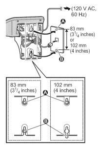
To remove the wall mounting adaptor While pushing down the release levers (①), remove the adaptor (②).
