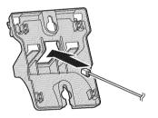
Tuck the telephone line cord inside the wall mounting adaptor (●). Connect the AC adaptor cord and telephone line cord (●).
