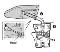
Insert the hooks on the wall mounting adaptor into the holes (a) and (2) on the base unit.
